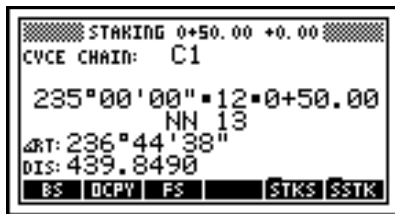
Figure 8-53 Stake the Next Station
