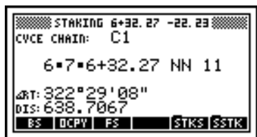
Figure 8-32 Station and Offset at Point 5
