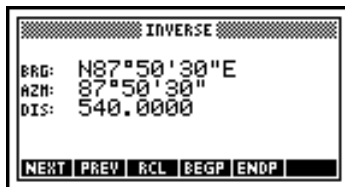
Figure 5-51 Inverting by Coordinates
