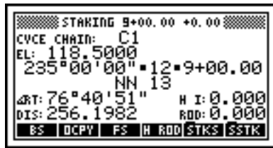
Figure 8-61 Elevation at Station 9+00
