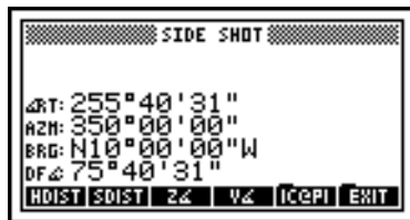
Figure 8-25 Azimuth from Point 5 to Point 6
