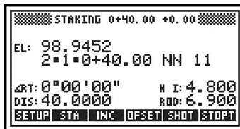
Figure A-68 Line Stakeout
