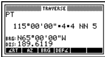
Figure 8-6 Bearing and Distance
