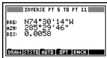
Figure 8-33 Inverse Point 5 to Point 11
