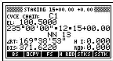
Figure 8-62 Elevation at Station 15+00
