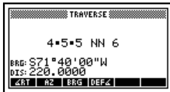
Figure 5-27 Traversing to Point 5
