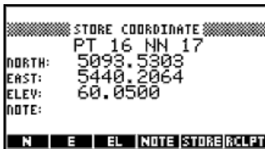
Figure A-72 Entering Point 16
