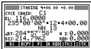
Figure 8-60 Elevation at Station 4+00
