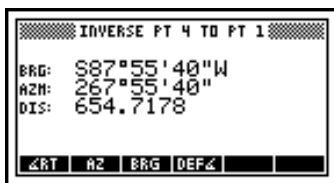
Figure 5-18 Inversing from Point 4 to Point 1
