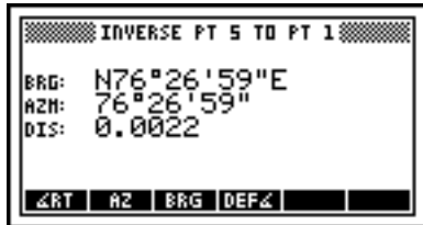
Figure 5-22 Checking the Error from Point 5 to Point 1
