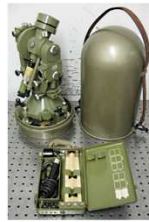
Wild T-3 theodolite, used for star observations and triangulation. 0.2" circle resolution; 0.1" estimation
