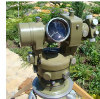
Kern DKM3 used for star observations and triangulation. 0.5" circle resolution; 0.1" estimation
