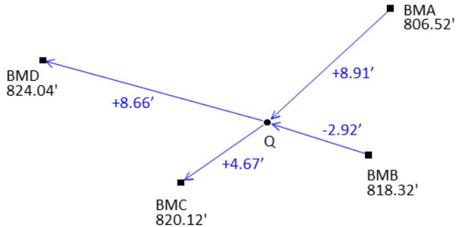
What is the most probable elevation of point Q? Determine to 0.001'.
